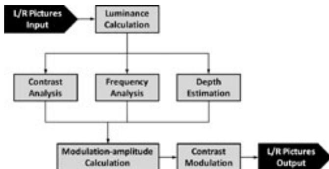
**FIGURE 2** — A block diagram of image processing.
