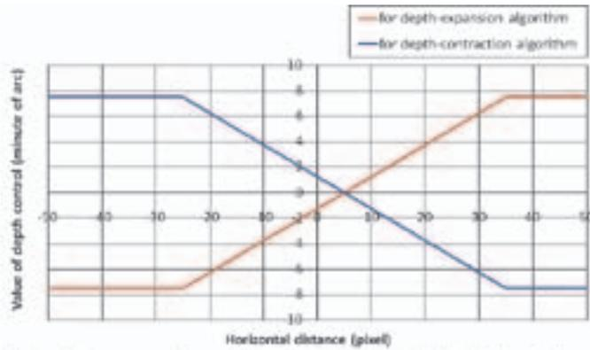
This graph is one example to explain how the depth-control value is determined. An actual relation will be calculated on the basis of an estimated depth of a picture. Positive and negative signs of the horizontal distance mean that the region is perceived in front of and behind the screen, respectively.
