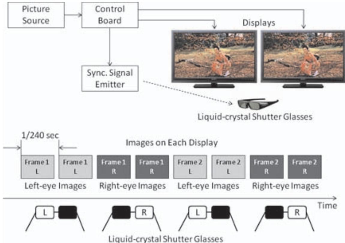
**FIGURE 4** — Display systems: connections between the displays and other equipment, and the operations of the displays and the shutter glasses.
